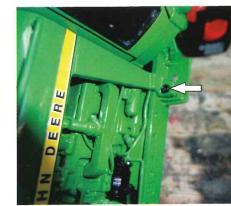
Two more are located under the battery boxes, meaning that they will have to come off. There will be a screw under each battery box that needs to be removed and the battery boxes will come off.
