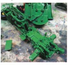
Now to reassemble. If you did a good job of keeping track of all of the screws, it is just a matter of reversing the process you used to disassemble the tractor, installing the fenders, then cab, then hood, making sure you reinstall the top steering shaft...then battery boxes and breaking the steering gear any more then
