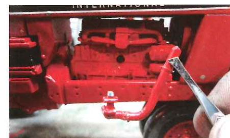
The carburetor and intake tube removed from the tractor and modified for the correct fit.
