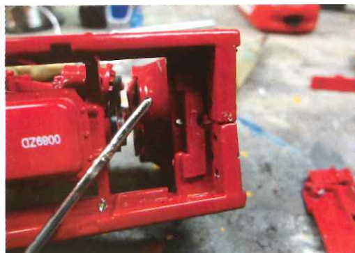
The steering shaft of the 1066 removed and straightened. Also the new location drilled a quarter of an inch back.
