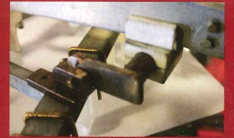
Here are some parts that were printed in bronze that I was able to grind to fit. The strength and ability to modify was second to none.
