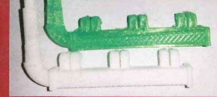
Here is a good example of two identical parts from different printers. The top green one was printed with a nylon weld-type printer and the lower white one with a resin type printer. The detail on the second one is tenfold better than the weld-type printer.
