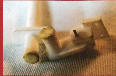
Here is one of the white flexible parts I had printed that broke. You can see I tried gluing it back together, with no success.
