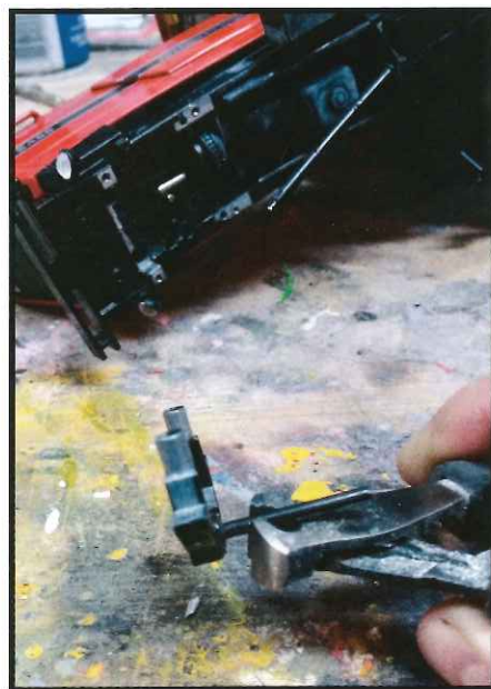
The underside of the 5488 with the mechanical-front-wheel-drive removed.
