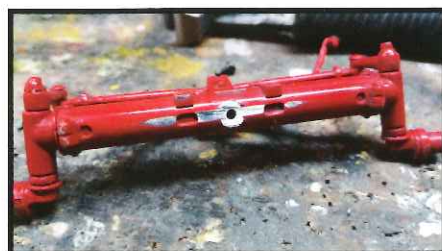
The 1468 front axle trimmed on the front for a better fit.
