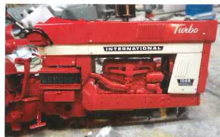
The hood test fitted.
