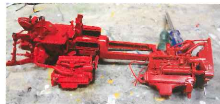
The engine removed from the 1066 chassis and chassis halves back together, with the 460 engine waiting for installation.
