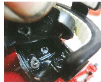
The seat cushion lifted from the seat frame of the 1066, exposing the screw that will need to be removed to take the seat off.
