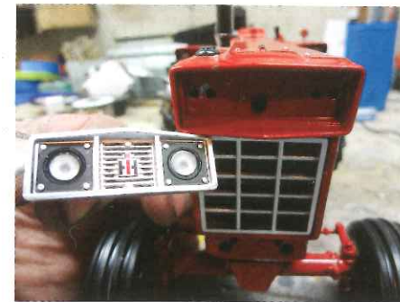
The upper grille and headlight bezel removed showing another screw.
