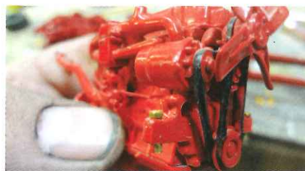
The front engine mount drilled with a 0.080 bolt install, ready to be mounted to the frame.
