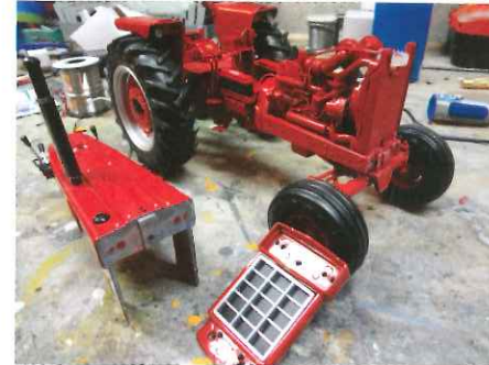
The grille and hood removed from the 1066.
