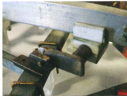
Some of the assembled parts. The gold parts are printed bronze.
