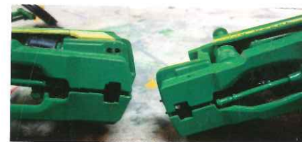
Both front ends removed. Notice the extra notch in the 730's chassis that will need to be removed.
