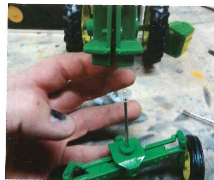
Casting halves spread and wide front removed from 720.
