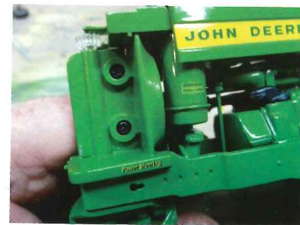
Nose cone removed from 720 exposing two screws holding casting halves together.
