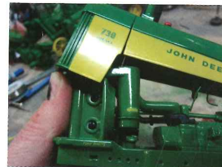
The 730's hood lifted up to get at the two screws holding the casting halves together.
