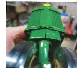
Bottom of the 730's chassis, showing the two screws holding the nose cone and hood on.
