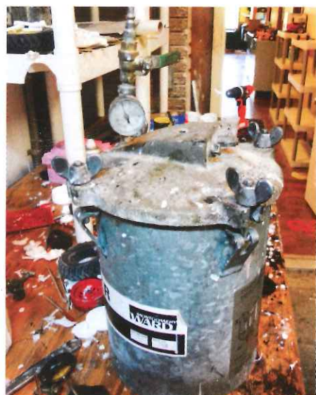
My pressure pot was built using a used three-gallon painter's pot.
