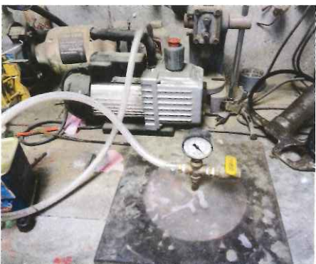
The pressure pot lid with the relief still intact but the paint hole plugged.
