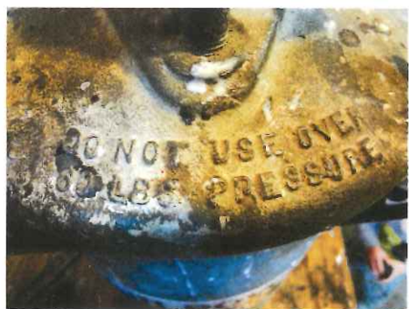
The lid of the pot clearly states, "Do not pressurize over 60 lbs."
