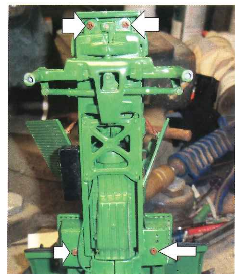
Looking at the underside, there are two screws under the weight bracket and two under the battery boxes. These must be removed.
