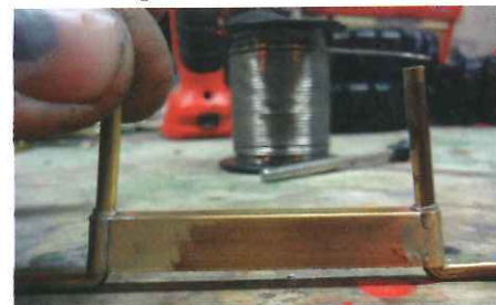
Test-fitting the steering knuckles in the axle tubes.
