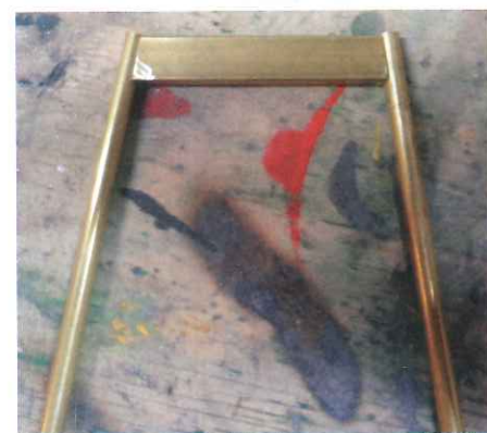
Spindle tubes fitted to the center beam.
