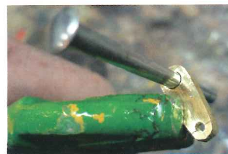
Tie rod ends being readied for shaping.
