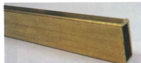
Center beam cut to length and tapered.
