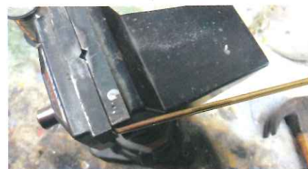
Steering knuckles bent tight in the vise.
