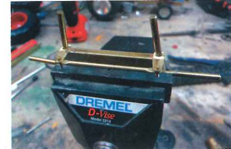
Tie rods being mounted to the steering arms.
