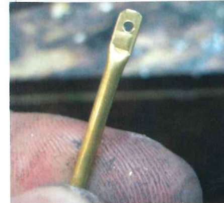
Tie rod end drilled and taped.
