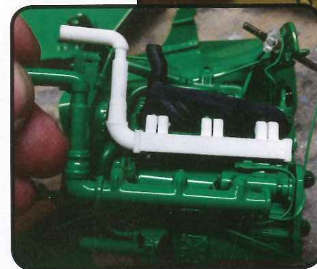
Here is the 5020 engine with the original intake manifold removed and the new 3-D printed manifold installed.
