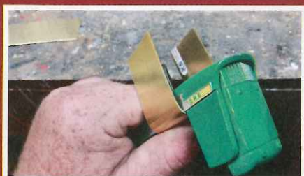
Using an old 4010 hood to bend the new 700A hood.
