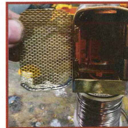
The front of the new hood with the grille cut to fit and brass square tubing soldered in place to hold the grille.
