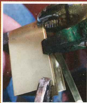
The new hood is soldered to the brass strip which was bolted to the underside of the hood. Also, the frame rails are installed and matched to the hood.
