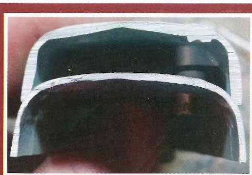
The underside of the hood needs to be trimmed to have a consistent thickness.
