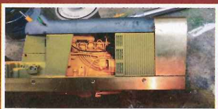
The new hood is soldered to the brass strip which was bolted to the underside of the hood. Also, the frame rails are installed and matched to the hood.
