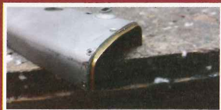
The brass strip is bolted to the underside of the hood.
