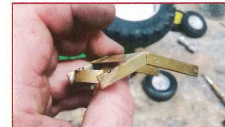
The beginning of the front weight bracket, with the notch cut out and bent, ready to be soldered.
