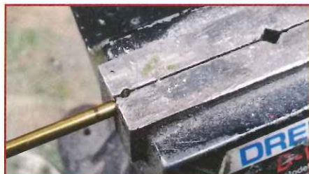
This is my Dremel vise with a 1/8-inch round bar clamped into the vise, ready to be drilled.
