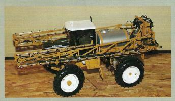
Dan Forbis, a custom builder from Riverton, Wy., logged 500 hours in creating this high-detailed 1:16 scale AgChem RoGator Model 854 field sprayer. The original sprayer had a 90-foot boom; therefore, this model is equipped with a 5 1/2-foot boom. The tank is constructed from wood, whereas, aluminum, copper and brass were used throughout. There are over 2,000 parts comprising this beautiful replica.
