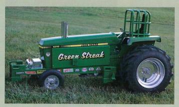
Dale Kolpin of Minnetonka, Minn., specializes in scratch building one-quarter scale puller tractors. This Green Streak puller has a fiberglass hood. The remaining parts, including the frame, are made from aluminum. This pro-stock replica is powered by a 35cc four-cycle Honda gas engine. The clutch and throttle are remote controlled. It weighs approximately 85 pounds.
